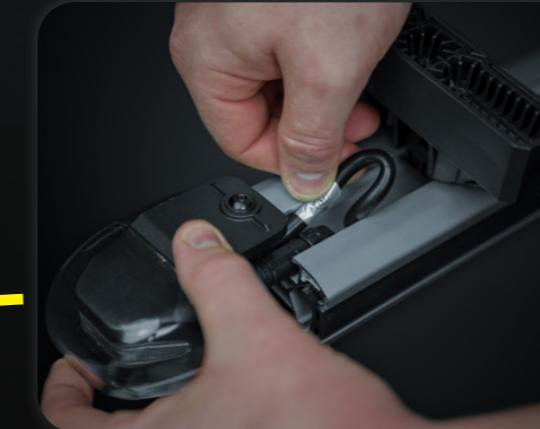
6. Mount the feet onto the rail by sliding them in from one side.
