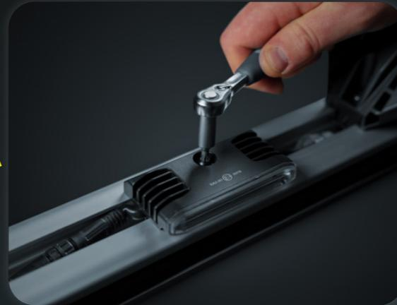
**11.** Secure the directional warning lights with a torque of 5 Nm.
