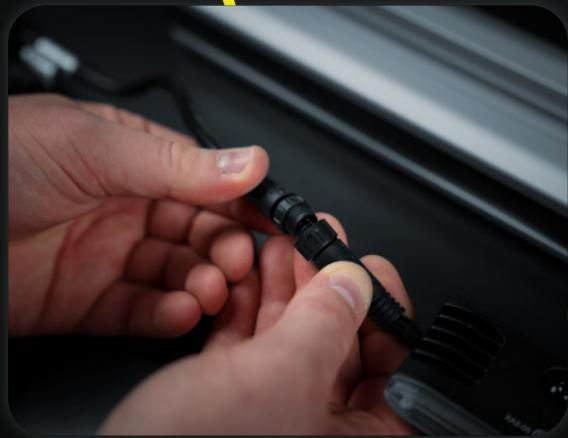
3. Connect all the cables together. Be sure to screw the connections tightly to prevent water from entering the connectors.
