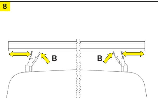
Measure so the roof bar is placed centered & tighten screw B on the back with 5Nm.
