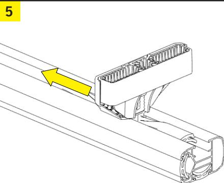
Apply soapy water on the lower cover strip to be able to easily slide the foot over it. Place the foot set about 10 cm in.
