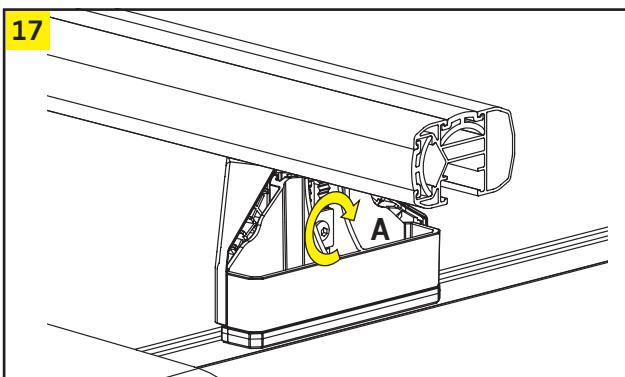
When the height is set correctly, tighten screw A with 5 Nm on all foot sets.
