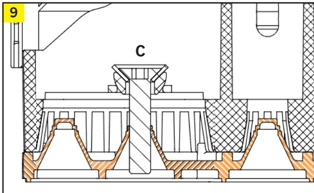
Check so the grommet is placed correctly and tighten screw C to 5 Nm.
