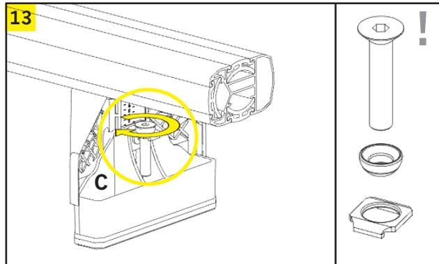
Take the screw, bushing & bracket through the foot & distance into the vehicle's fix-point.
