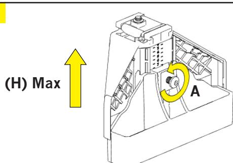
Loosen screw A on the front to raise the foot to the
