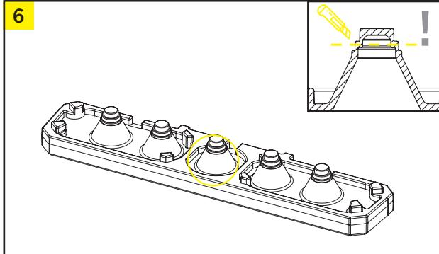
Prepare the distances & cut the bottom marking on the grommet in the center. Make sure the grommet follows the curvature of the roof as this may differ on some models
