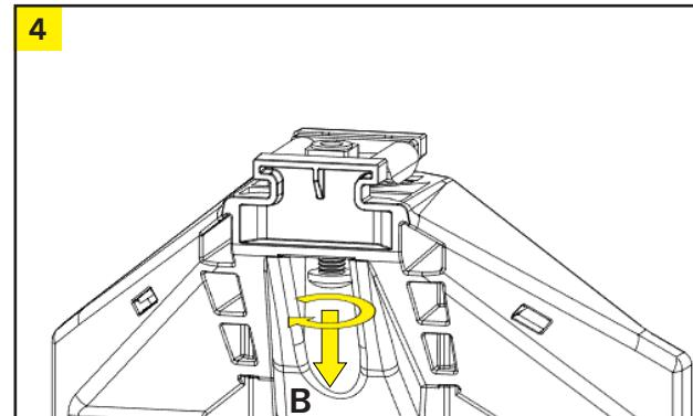
Loosen screw B on the back until flush with the nut on
